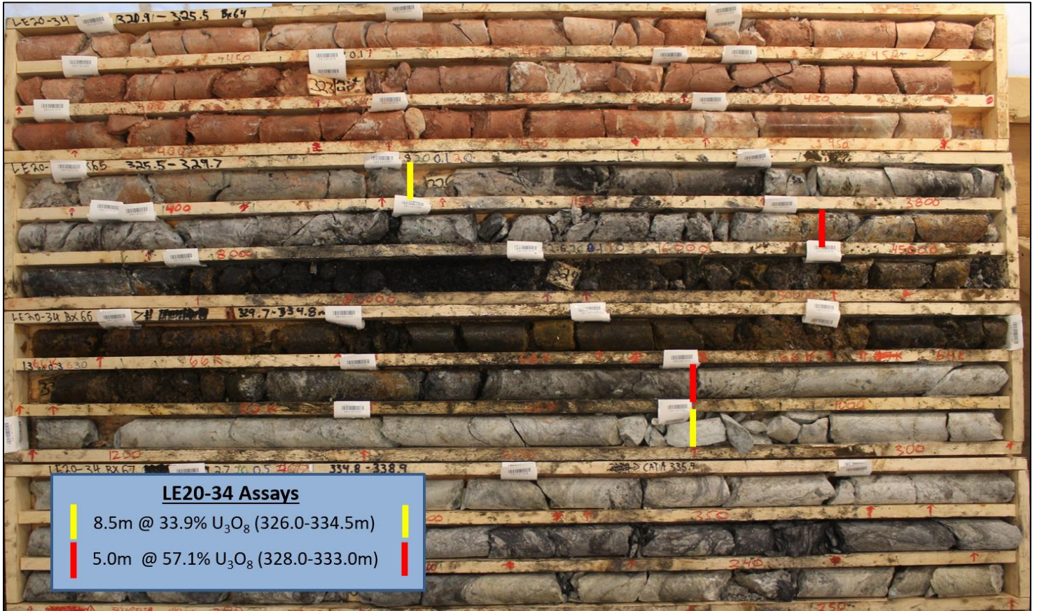
Figure 4 – Drill Hole LE20-34 Core Photo of Mineralization
